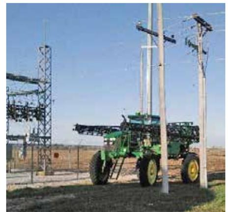
A place to park? It may be convenient for the sprayer operator, but parking between a substation and several power poles is risky. If the booms were accidentally extended, they could easily conduct electricity and become a deadly hazard.
